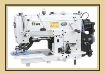
8) BUTTON ATTACHMENT MACHINE ?This is used in attaching buttons to the garments.
