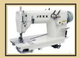
7) BUTTON HOLER MACHINE ?This is used in making buttonholes on garments.
